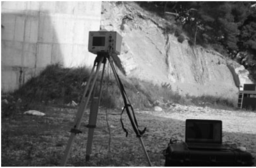
Figure 2. Terrestrial laser scanner ILRIS-3D-ER on pilot site “Žnjan 1”.
