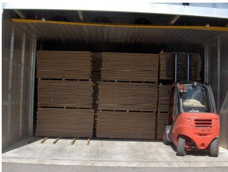
Figure 1. Conventional (aluminium/concrete) wood drying kiln interior (photo: Klarić)
