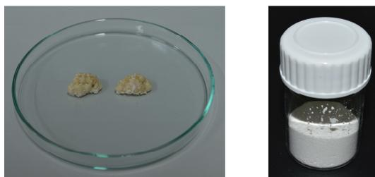
*Figure 4. Deposit sample before milling (left), and after milling (right) (photo: Klarić)*
