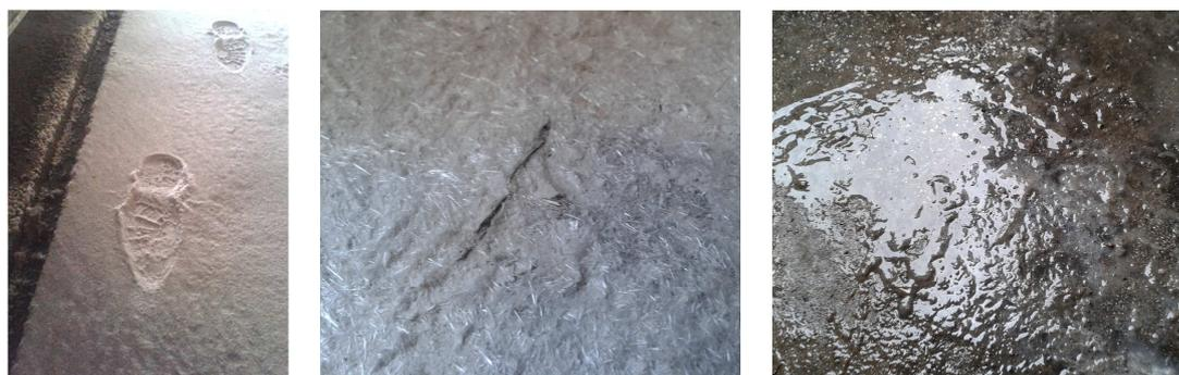
Figure 9. Powdery deposits (left, middle); slimy and goeey mash (right) (photo: Pervan)
