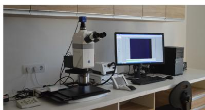
*Figure 5. Axio Zoom V16, Zeiss. LDG laboratory (photo: Klarić)*
