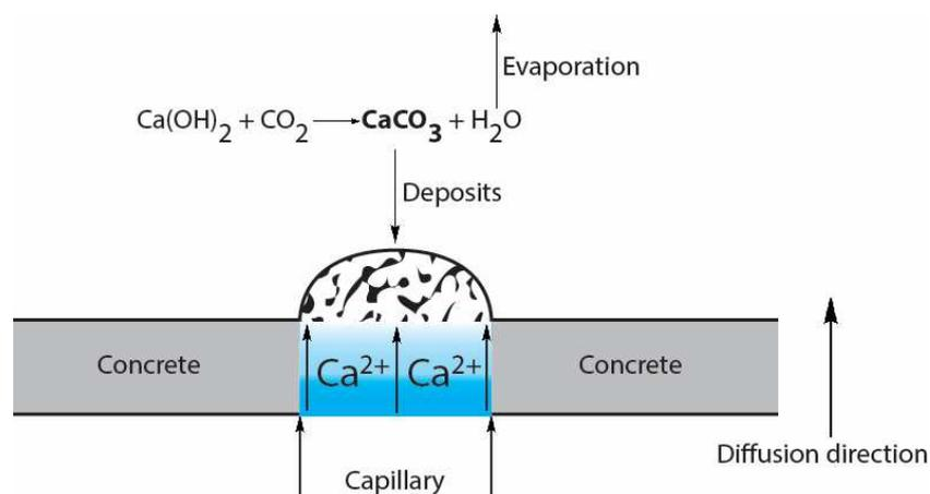
*Figure 7. Schematic diagram of deposits formation on concrete surface (simplified according to Kresse, 1987)*
