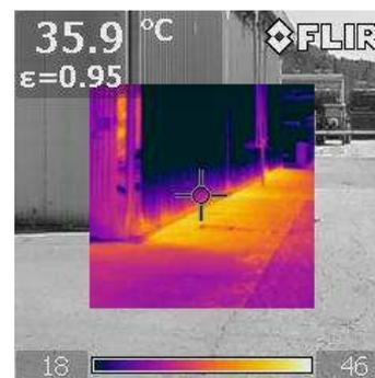
Figure 2. Infrared image of conventional wood drying kiln exterior, showing condensate and heat flow (photo: Klarić)
