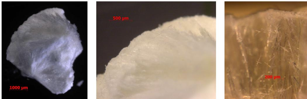
*Figure 6. Efflorescence sample, magnification 12.5x (left), 32x (middle), 80x (right) (photo: Klarić & Španić)*
