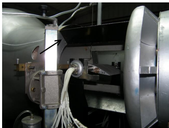
Figure 2 – Airfoil in the test section of AT-1 wind tunnel
