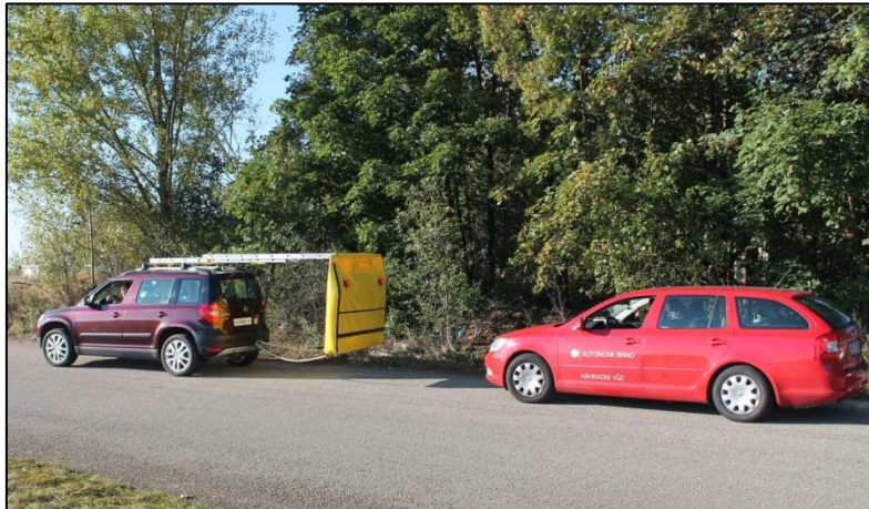
Figure 2 – Simulator with flexible crash barrier on vehicle Škoda Yeti and test vehicle Škoda Octavia Source: authors
