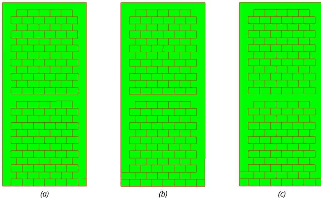
**Fig. 14** Crack initiation and propagation for  $a_g=3.0 \text{ m/s}^2$ : (a)  $t=1.97 \text{ s}$ ; (b)  $t=7.12 \text{ s}$ ; (c)  $t=12.00 \text{ s}$
