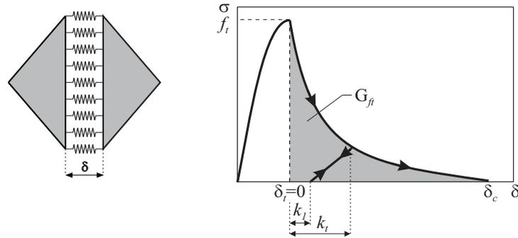
**Fig. 2** Strain softening curve defined in terms of displacements
