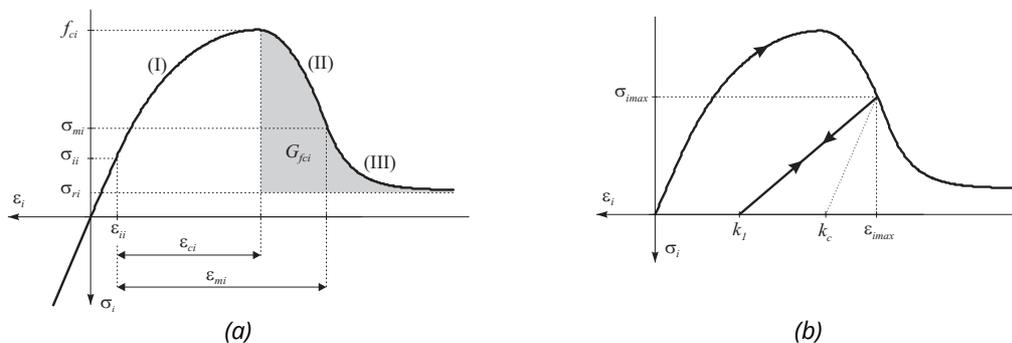
Fig. 5 The material model in a unit: (a) Hardening/softening law for compression; (b) Cyclic behaviour in compression [24]
