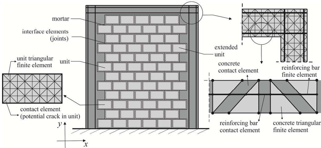
**Fig. 1** Discretization of a confined masonry structure
