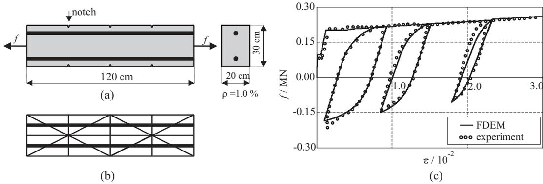
**Fig. 7** Beam characteristics: (a) specimen for cyclic loading test; (b) finite element mesh and reinforcing bars of the beam; (c) force - average axial strain relation
