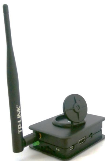
Figure 4 – Camera and Bluetooth detector built during this project.
