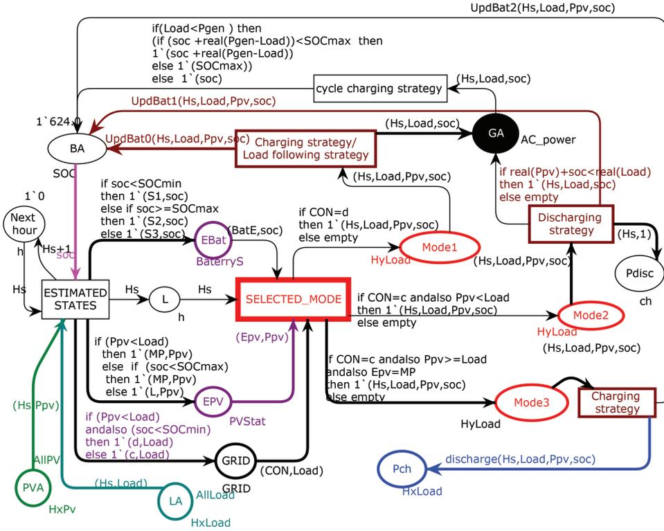
Figure 4. The CPN model for the cooperation process of the MAS.
