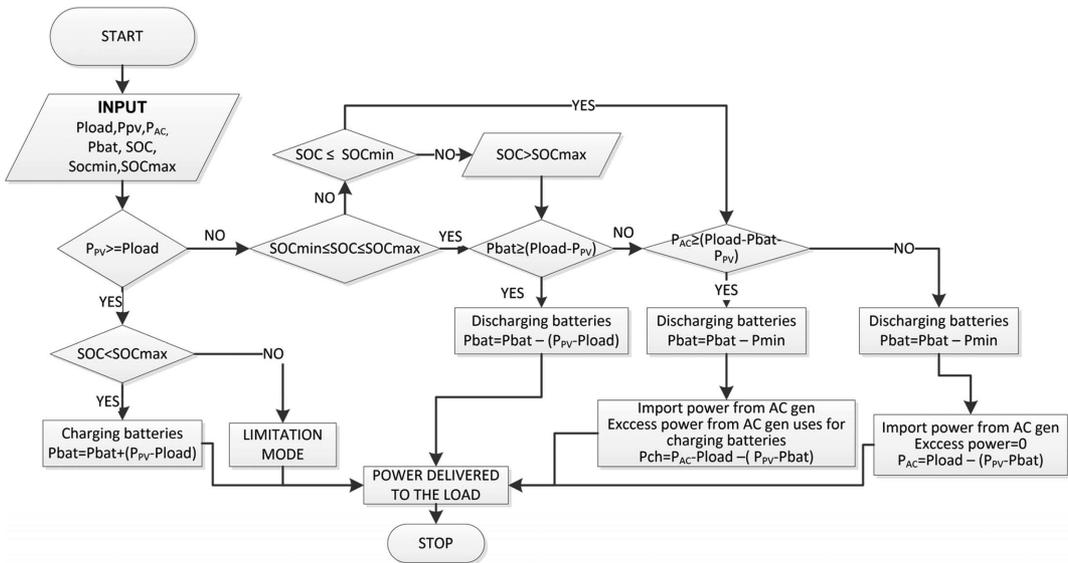
Figure 3. Flow chart of power management on the ship.
