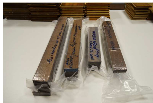
Figure 8. Vacuum-sealed elements (photo: Klarić)
