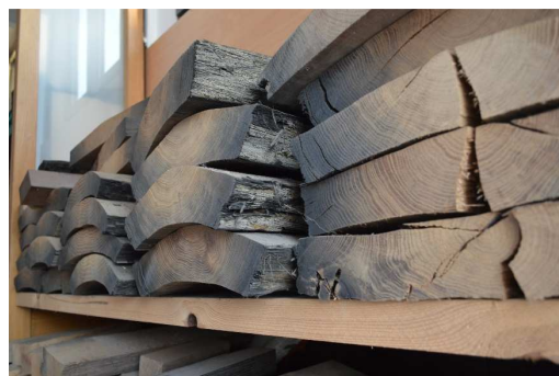
Figure 4. Abonos shrinkage and cracks (photo: Klarić)
