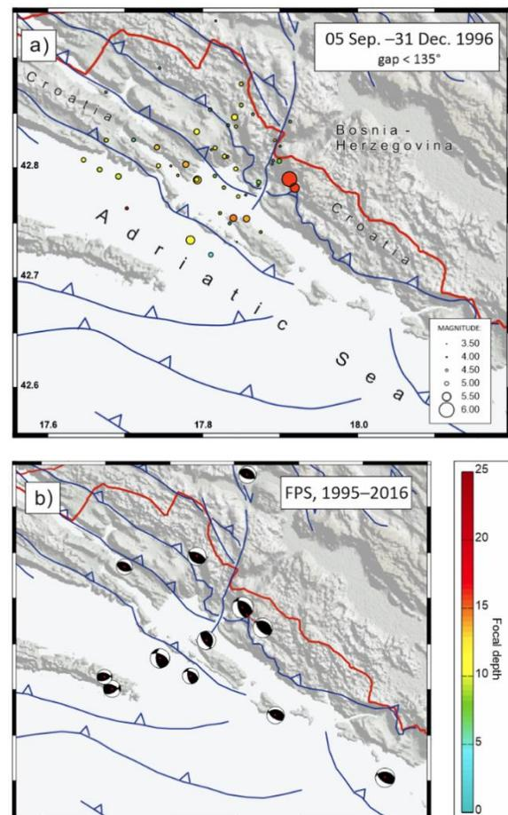
**Fig. 2.** a) Reliably located epicentres of the 1996 Ston–Slano earthquake sequence. b) Fault-plane solutions (FPS; lower hemisphere stereographic projection, compressive quadrants are black) for the earthquakes in the period 1995–2016. Surface traces of faults (after Raić et al., 1980; Tomljenović et al., 2009 with references therein) are shown by blue lines, with barbs on the hanging wall of reverse faults.
