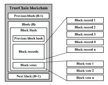
Figure 2. The TrustChain blockchain architecture
