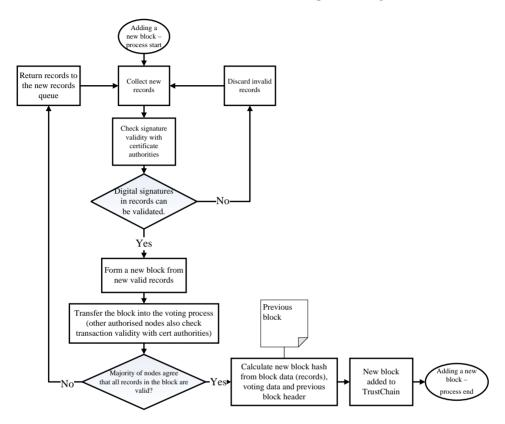
Diagram 2. Adding a new block to the TrustChain
