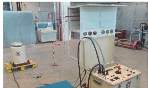
Figure 5. Short-duration power frequency withstand voltage test of the prototype
