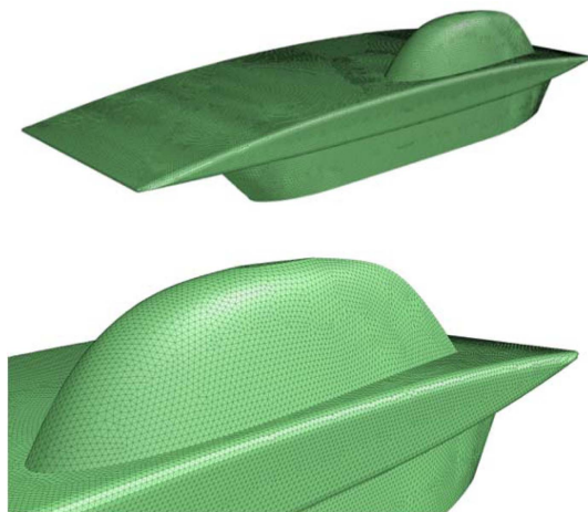
Figure 5. Details of the geometrical discretization of the vehicle body.
