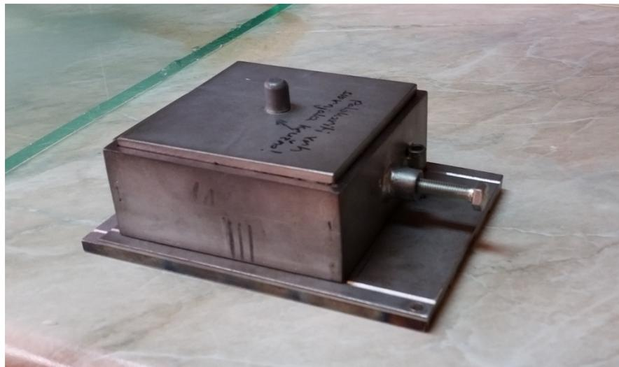
**Figure 5:** Adaptation of direct shear cell for measuring friction angle on steel
