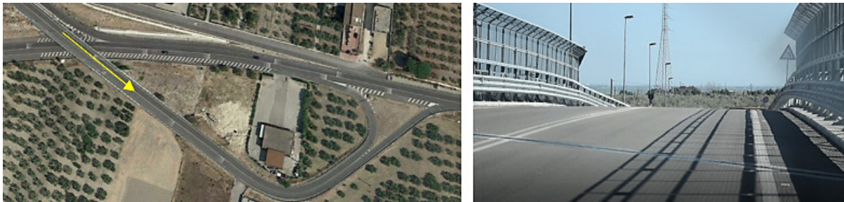
Fig. 11. Section 5 – Poor Coordination of Horizontal and Vertical Alignments
