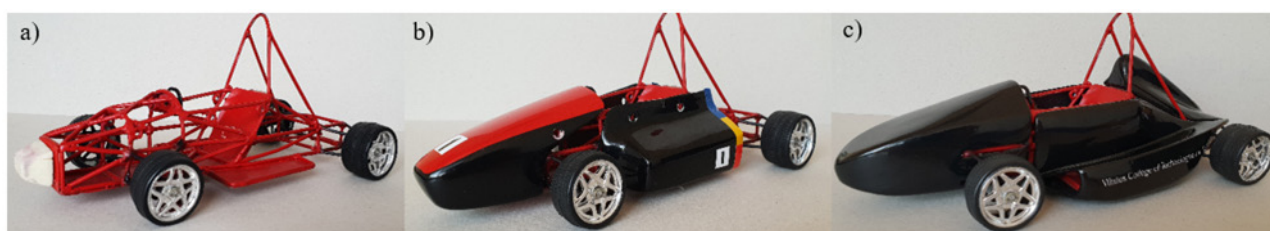
Fig. 6. “Formula Student” model prepared for measurement in wind tunnel: a) – without the body; b) – with old body; c) – with new designed body
