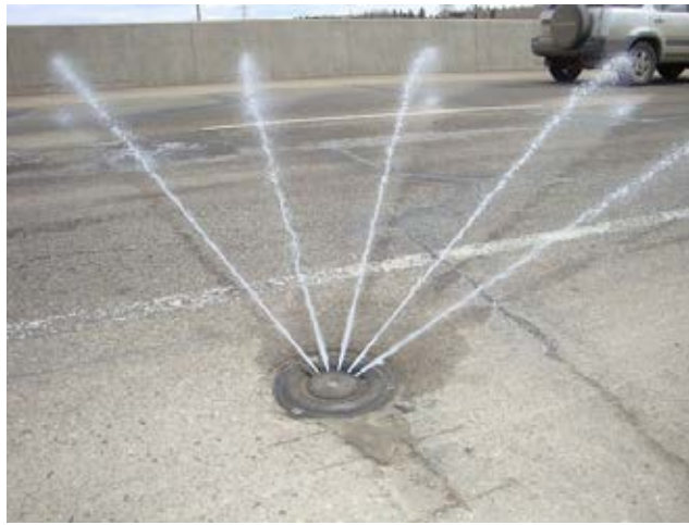
Fig. 10. Spray Nozzle of Detecting and Preventing System Source: Rock to Road, 2015
