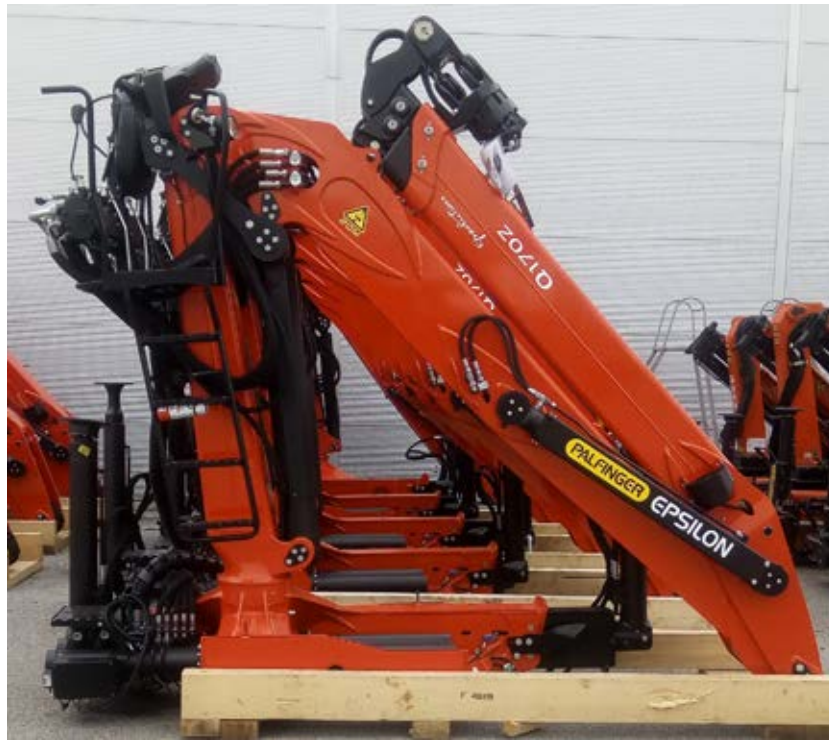
Fig. 3. Hydraulic lifting device PK_6501_HP Source: authors
