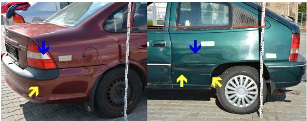
Fig. 3. Correspondence of damage vehicles Opel Vectra and Daewoo Nexia
