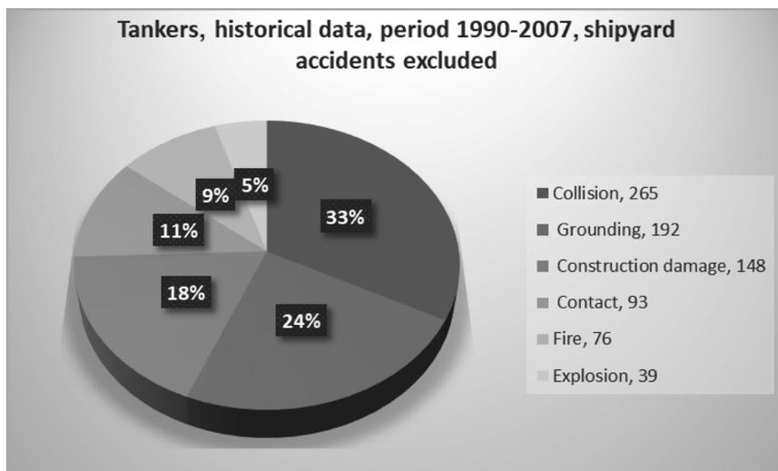
Figure 1 – Accident categories of tankers larger than 60.000 DWT [9]
