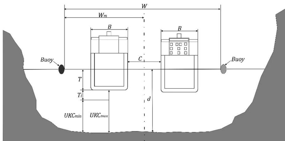
Figure 2 – Geometric features of waterway (Source: Authors)
