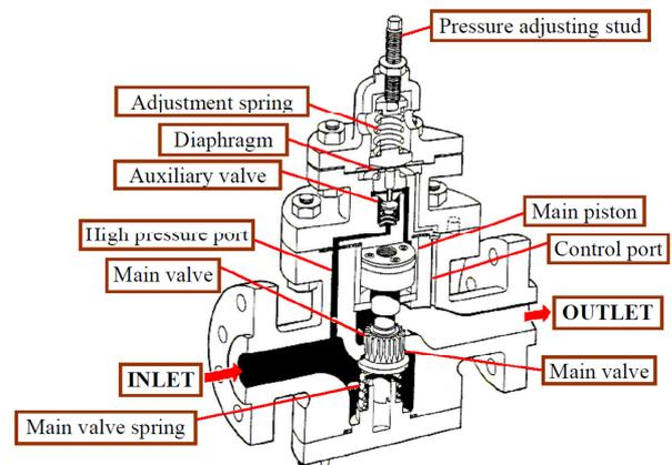
**Fig. 1.** Analyzed steam pressure reduction valve intersection [9]
